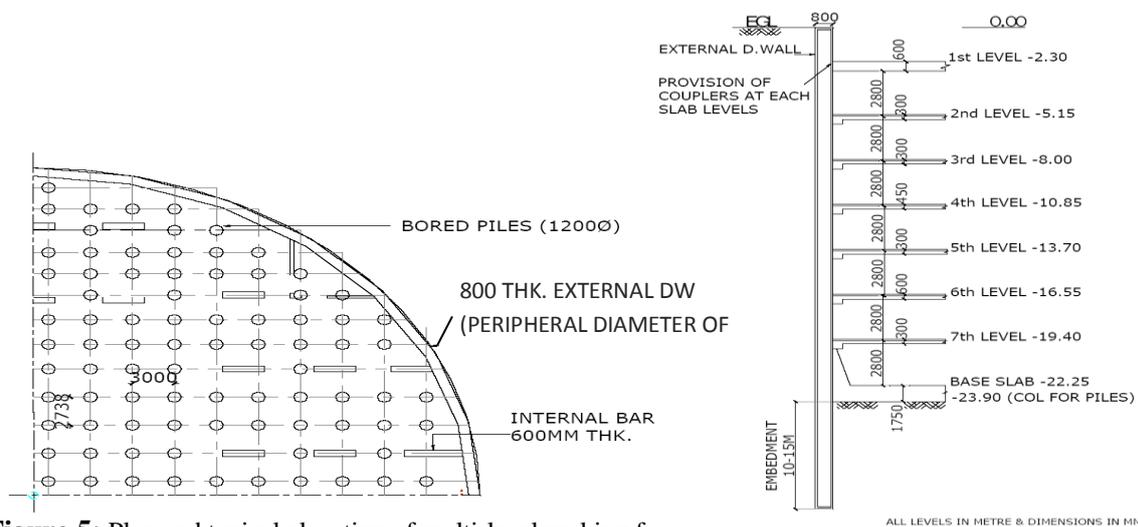
**Figure 5:** Plan and typical elevation of multi-level parking facility
