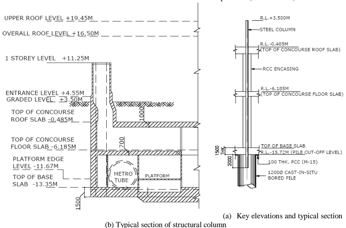
**Figure 6:** Metro station elevation and structural column details
