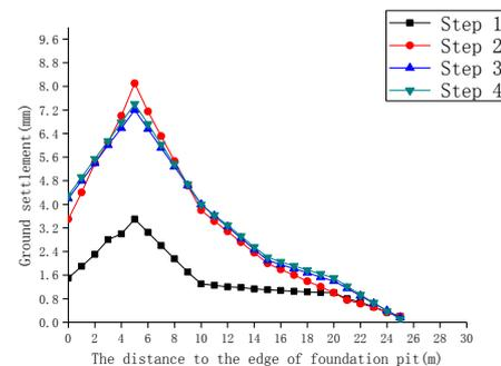
Figure 6. The curve of ground settlement.
