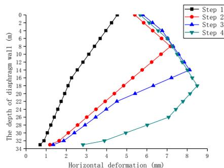
Figure 11. The curve of the horizontal deformation of retaining structure
