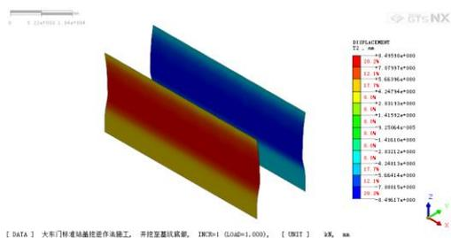
Figure 10. The horizontal deformation of retaining structure (Step 4)
