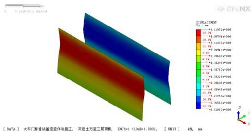
Figure 9. The horizontal deformation of retaining structure (Step 3)
