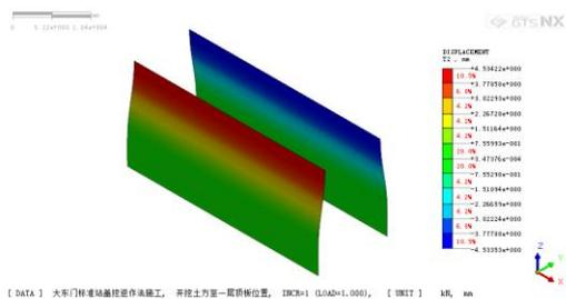
Figure 7. The horizontal deformation of retaining structure (Step 1)
